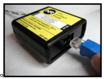
If the NTMS is powered up, and the CAT5E cable connection is made correctly between the DCP and the NTMS, the yellow LED on the DCP will illuminate and blink quickly ten times.
