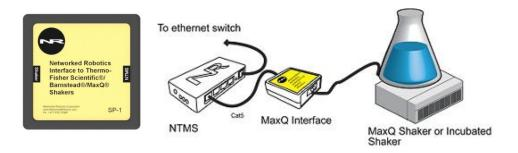
The MaxQ line has both digital and analog versions of each model. This product is compatible with the digital-version models only, all of which have serial data ports for data output. Digital versions comprise the E-series and have "SHKE" model numbers. The SHKE 420, 481, 2000, 4000, 4450, 5000, and 7000 models support the use of this product. This interface is not appropriate for use with the A-series (analog) versions of the MaxQ line.
