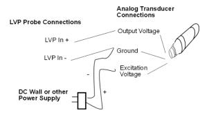
Transducer output is connected to the Low Voltage Probe as shown below:
