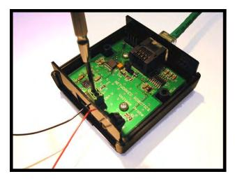
Attach the negative or ground wire of the sensor's output voltage to the screw terminal labeled (IN-) on the Voltage Probe board. This is the leftmost pin when facing the LEDS.
