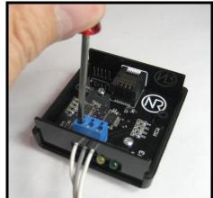
Replace the cover and its screws to close the DCP. Then use the provided CAT5E cable to connect the DCP to any of the four probe ports on the NTMS. If needed, you can use a longer length of CAT5 cable. The maximum distance, however, should not exceed 100 meters.
