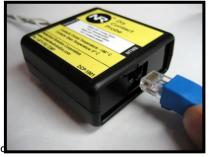
If the NTMS is powered up, and the CAT5E cable connection is made correctly between the DCP and the NTMS, the yellow LED on the DCP will illuminate and blink quickly ten times.
